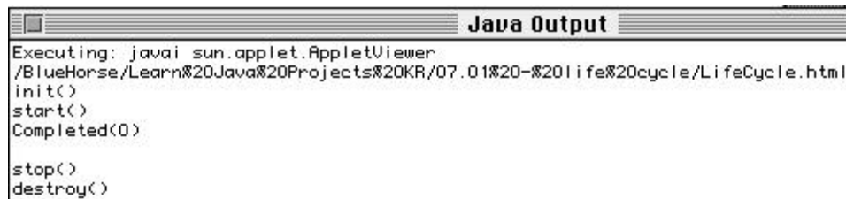
Figure 7.9 Closing the Applet Viewer so that the applet goes away. (The applet completes the rest of its life cycle methods by invoking stop() and destroy() )
